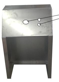
Before drilling holes to mount dials and steering system make sure they are properly laid out.
